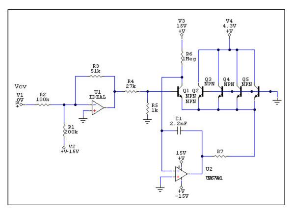
The above circuit is the current sink that generates labc for each of the OTAs. The 4 NPN collectors (Q2,3,4,5) are labc1, 2, 3, and 4. The resistor R7 (not given a value yet) is used to limit the maximum current of the current sinks (more on this later). First we find the output voltage of the opamp (U1) as a function of the Vcv control voltage:
