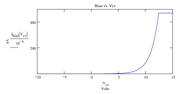
Yes, I did cheat and manually clip the plot at 470uA. One other point to note is that a normal 0..+5V control voltage cannot sweep the filter across it's entire audio range. If this is wanted, then a smaller input resistor on the U1 opamp would achieve this. Perhaps for the second CV input. The first would be labeled 1V/oct and the second could be labeled CV1.
